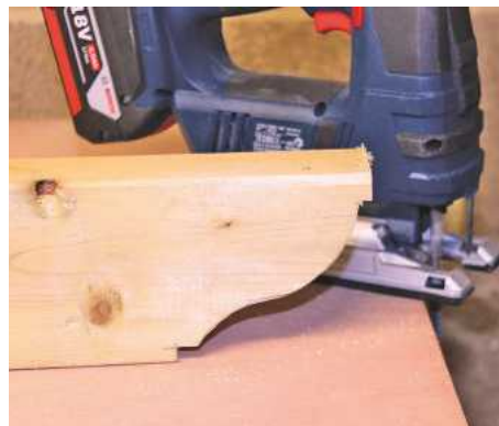
▲ Curved bracket work should be part of the remit, and the cut should be square
